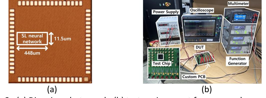
**Fig. 2.** (a) Die microphotograph, (b) test environment for proposed sound localization neural network
